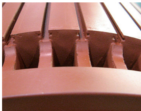
Fig. 2 Slots of the rotor of the prototype motor
