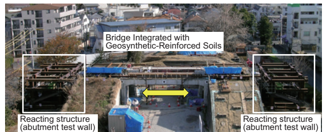
Fig. 2 Alternating horizontal loading test set up
