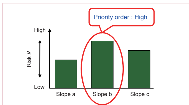
Fig. 2 Results of an experimental risk calculation for falling stone incidents
