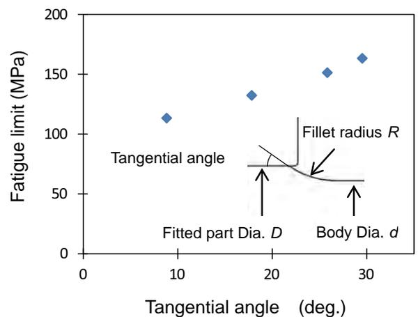
Fig.1 Relationship between fatigue limit and tangential angle  $\theta$
