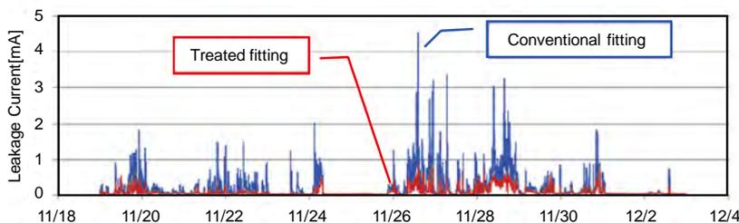
Fig. 2 Measurement Results of Leakage Currents
