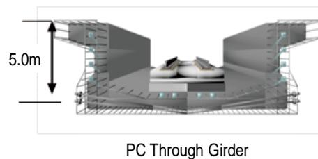
Fig. 2 Cross-section shape of test specimen
