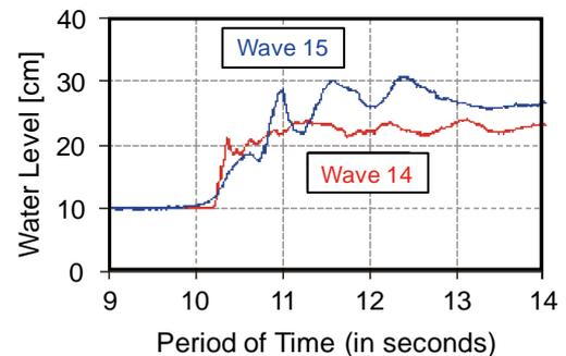
Fig. 1 Tsunami waveforms used for test
