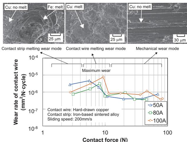
Fig.2 Wear rate and wear surface of contact wire
