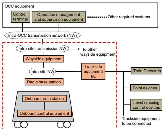
Fig.1 Overview of Structure of Train Control System Using Radio Communications
