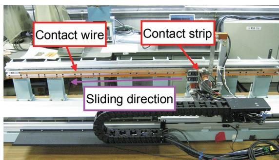
Fig.1 Linear wear test apparatus
