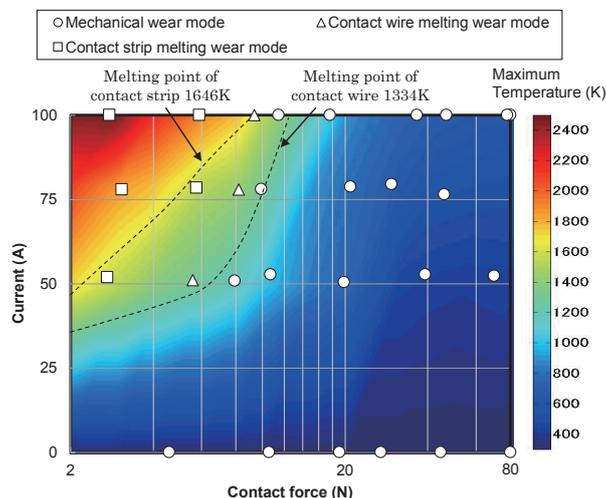
Fig.3 Correlation between wear mode and maximum contact temperature
