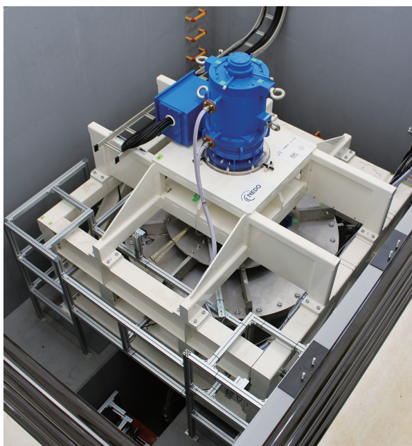
Fig.1 Superconducting Flywheel Energy Storage Unit
