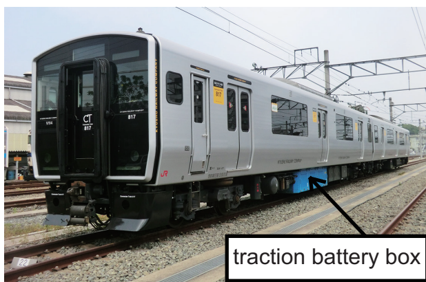
Fig.1 Battery-powered and AC-fed Hybrid EMU (test train)
