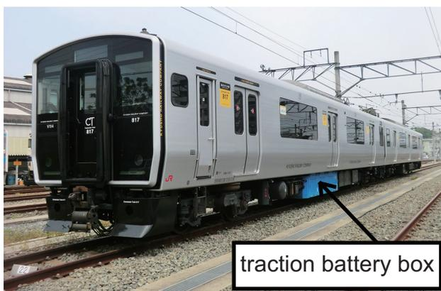
Fig.1 Battery-powered and AC-fed Hybrid EMU (test train)
