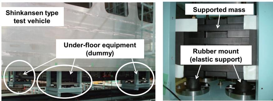
Fig.1 Setting of the dummy under-floor equipment to the carbody
