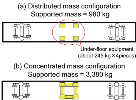
Fig.2 Loading conditions of the under-floor equipment
