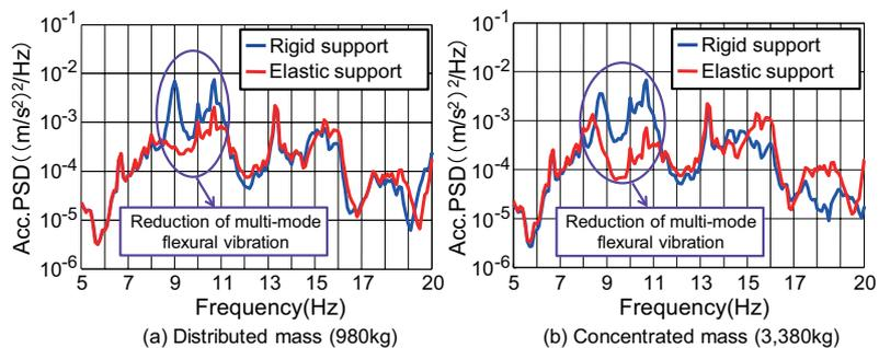
Fig.3 Acceleration PSD on the carbody floor measured under the central window (Simulated running excitation corresponding to 240 km/h)
