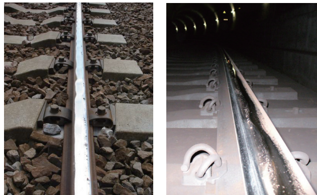
Fig. 2 Examples of rail corrugation (left: low rail on ballasted track; right: high rail on ballastless track)
