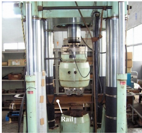
Fig. 9 Bending fatigue test situation
