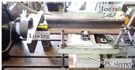
Fig. 13 Setup of rail creep resistance test
