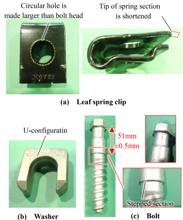
Fig. 4 Components of the proposed rail fastening system
