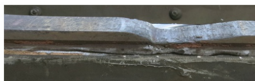
Fig. 2 Example of localized wear of contact strip
