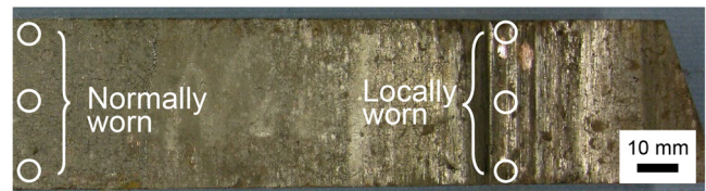
Fig. 10 Points of Raman spectroscopic analysis for actual contact strip
