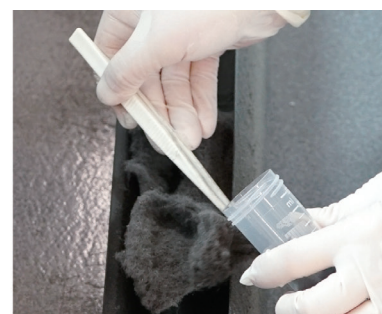
Dust collection by scraping
