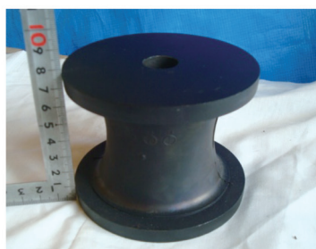
(c) Rubber mount (elastic supporting device)
