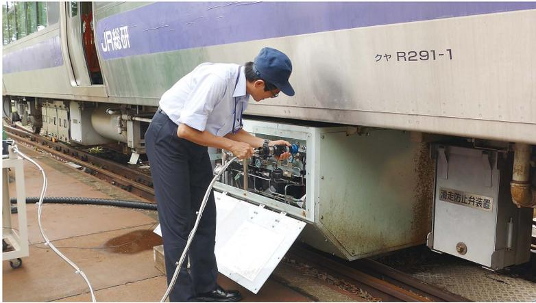
Filling up the tank on the RTRI's full-scale prototype vehicle with hydrogen
