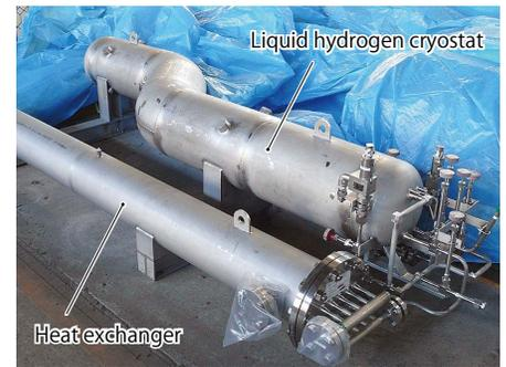
Prototype of liquefied hydrogen storage container (in 2012)
