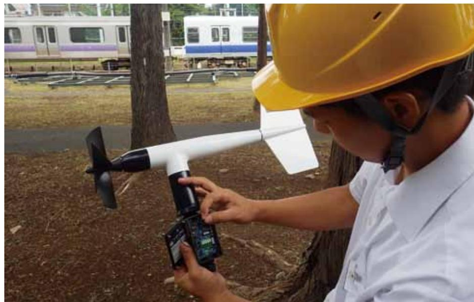
Wind observation is indispensable to creating hazard map system for strong wind. In order to validate the simulation result for meteorological phenomena, we measure the velocity and the direction of wind which blows in the target areas by propeller anemometers.
