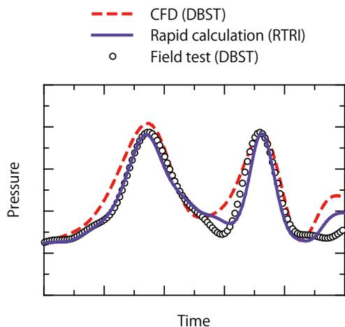
**Fig. 1: Comparison of the MPW prediction results**
