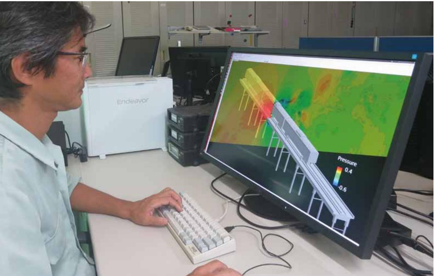
**This screen shows a pressure distribution around the center of train. The higher pressure region (red colored) is on the upper stream side of the train. Numerical simulation is expected to become an effective method to acquire detailed data from an unsteady three-dimensional flow field.**
