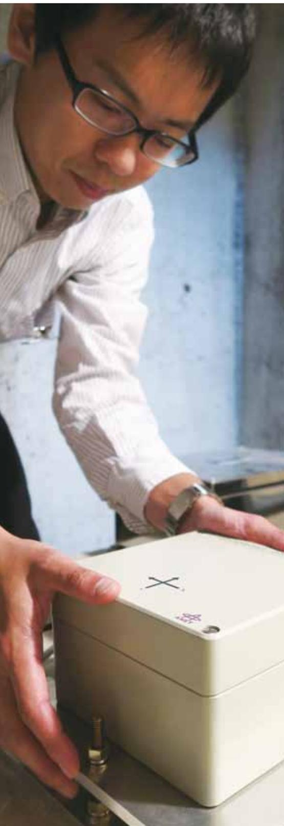
In addition to having functions to issue a warning after detecting large tremors, each seismometer has a specific function called a P-wave warning function, which can issue a warning by analyzing preliminary tremors (P-waves) that arrive prior to large tremors (S-waves). The greatest feature of the earthquake early warning system lies in its ability to issue P-wave warnings.
