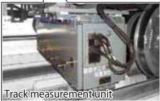
Car body-mounted track measurement device
