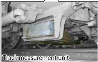
Bogie-mounted track measurement device
