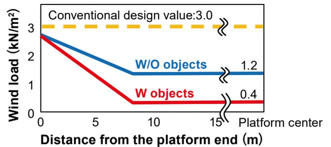
Load or pressure need to be considered in design (Platform screen door support)
