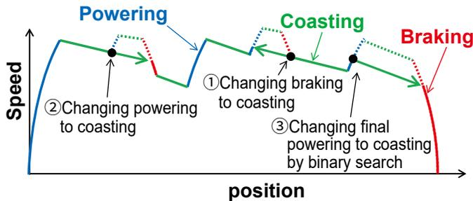
\* After the shortest speed profile (dotted line) has been created, a speed profile for energy consumption estimation (solid line) is created by inserting coasting lines one by one to meet the designated running time.
