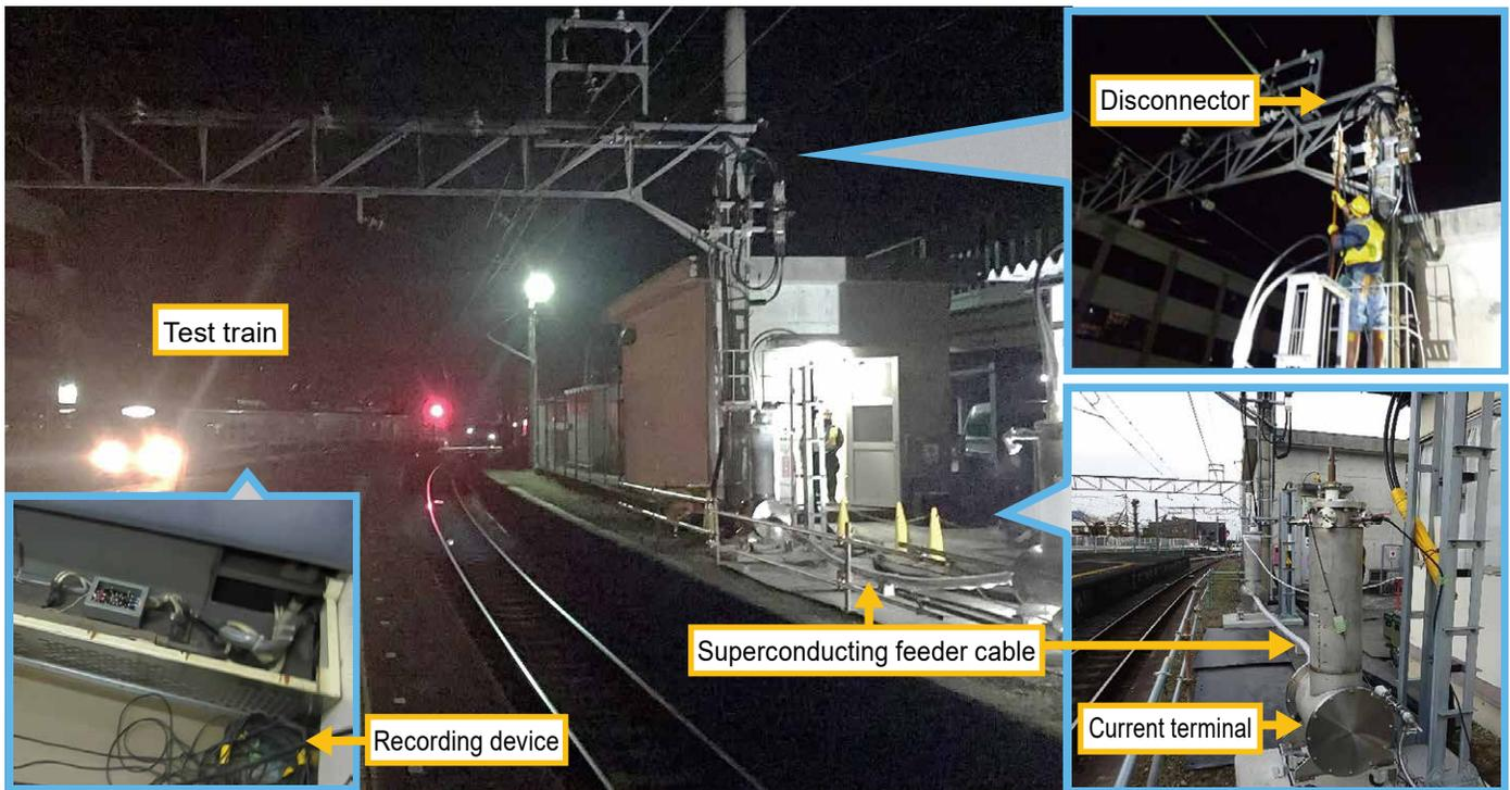
**Superconducting feeder cable connected to a track**
