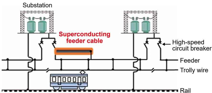
Superconducting feeder cable introduced to a feeding system (Connecting part of substations)
