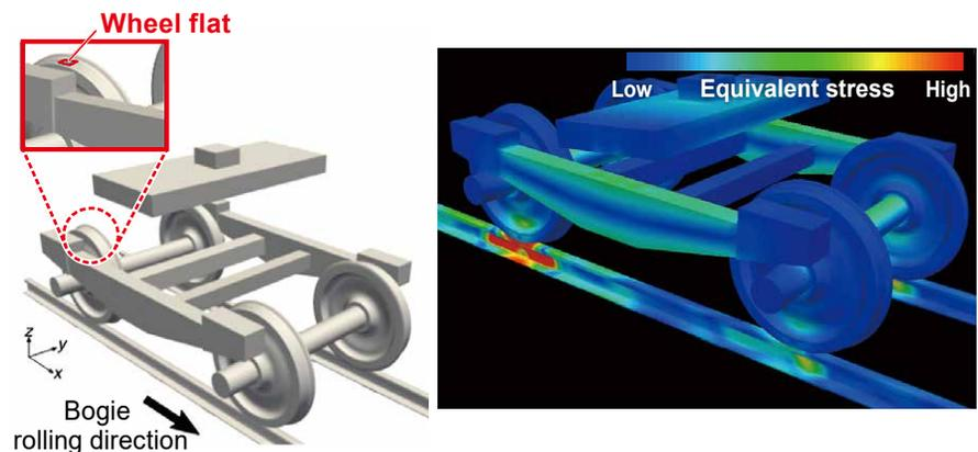
**Simulation example of a bogie using a wheel with tread flat damage**
