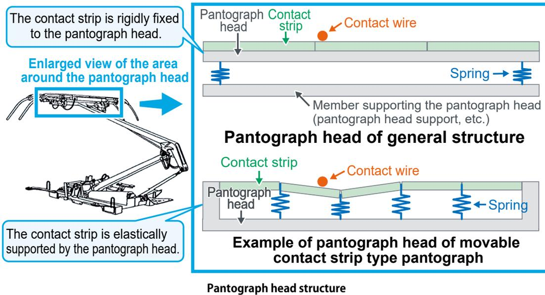
force. While the vehicle is at a standstill, the pantograph is in contact with the contact wire with a nearly constant contact force (50 to 60 N). However, during running, the contact force fluctuates due to the effect of, for example, the height difference of the contact line between the supporting points and the middle part of
