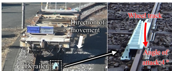
Fig. 12 Appearance of installation of the derailer
