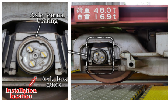
Fig. 4 Installation locations for contact sensors
