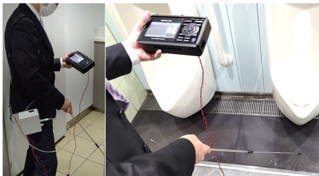
Fig. 2 Use of high-sensitivity \text{NH}_3 measuring instrument in men’s station restroom
