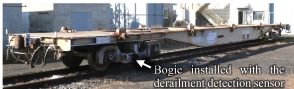
Fig. 11 Appearance of vehicle used for derailment detection test
