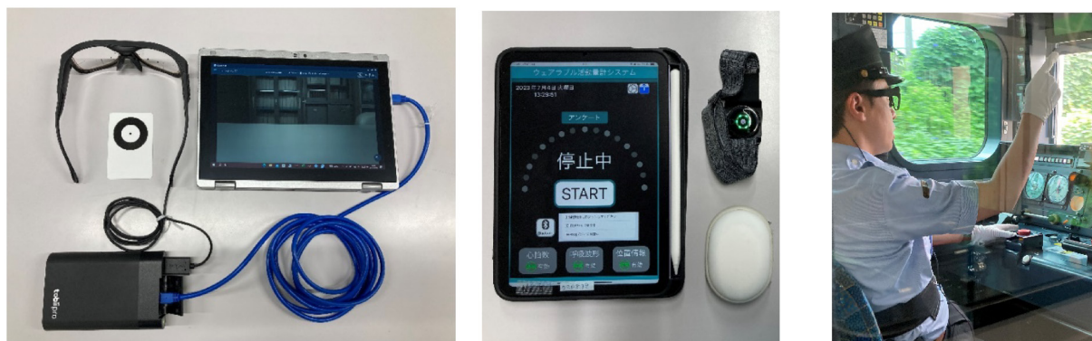
Fig. 7 Measurement equipment (left: eyeglass-type sensor, center: physiological measurement system CHET) and measurement during operation (right)
