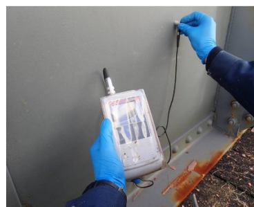
Fig. 1 Measurement of coating thickness using an electromagnetic coating thickness gauge
