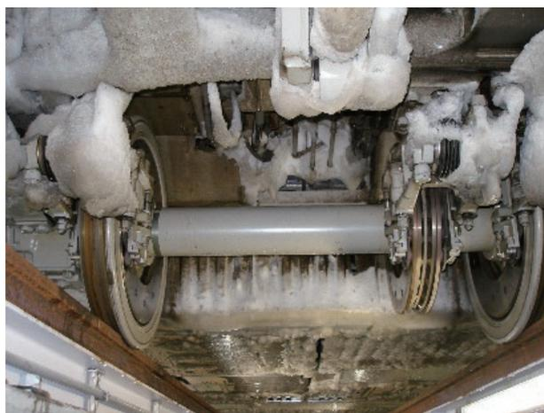
**Fig. 1** Railway vehicle bogie with snow accretion
