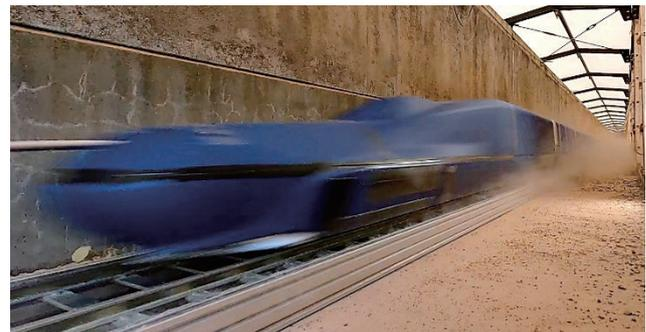
**Fig. 3 Vehicle model running experiment using artificial snow**
