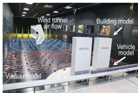
Fig. 2 Wind tunnel test
