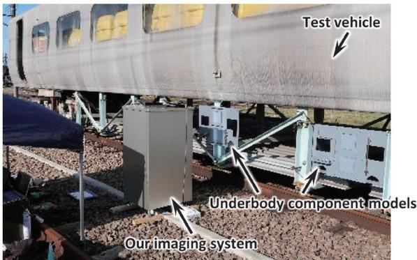
**Fig. 8 Image capture test simulating underbody equipment anomalies**
