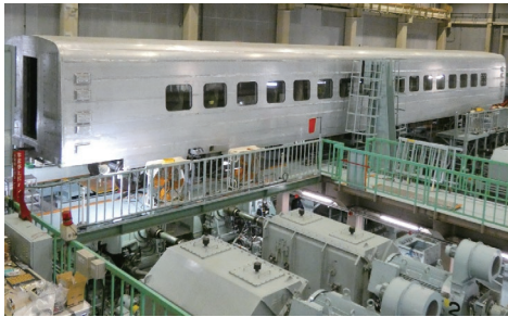
Fig. 11 Testing with a Shinkansen-type test vehicle in the rolling stock testing plant at RTRI
