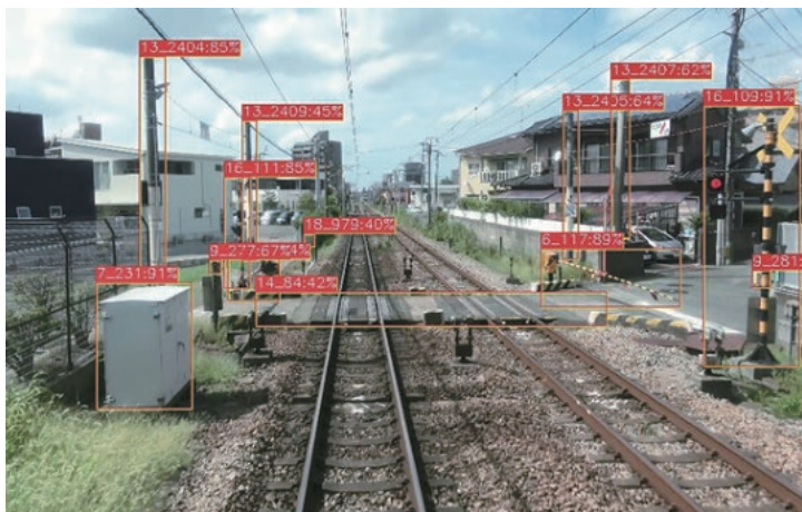
Fig. 2 Example of equipment recognition result
