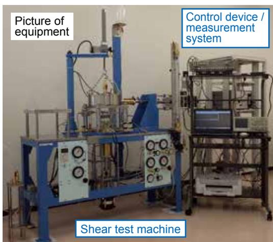
Fig. 2 Hybrid ground response test equipment and schematic overview
