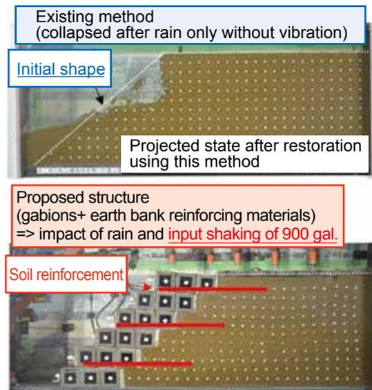
Fig. 2 Functional verification testing increased resistance to rain fall and earthquakes
