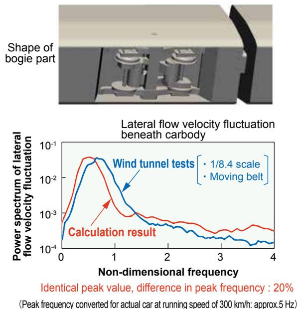
Fig. 2 Comparison of fluid analysis and wind tunnel test
