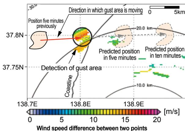
Fig. 1 Detection of gust area in the upper air from meteorological radar readings
