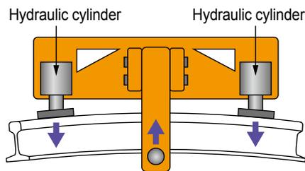
Fig. 2 Bending upwards the repaired part of the rail by hot correcting
