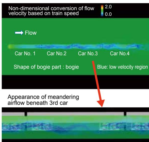
Fig. 1 Fluid analysis considering bogie
