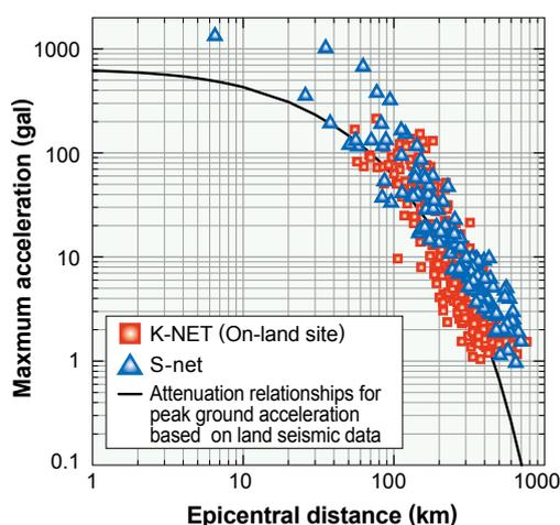
Fig. 1 Comparison of observation data with attenuation relationships
