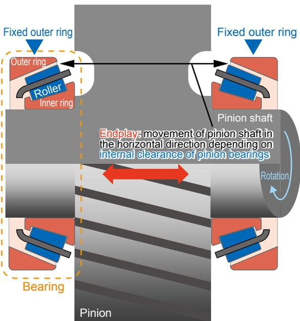
Fig.1 Pinion shaft bearing endplay
