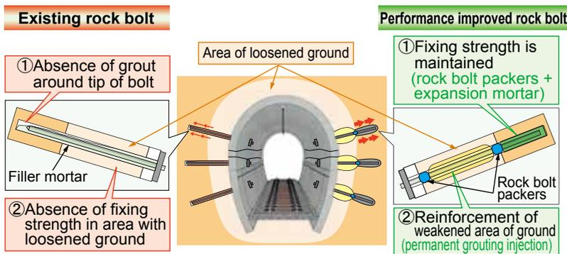
Fig. 1 Comparison with existing type of rock bolt
