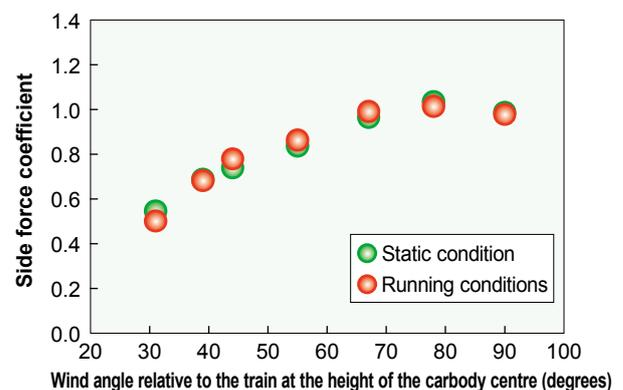
Fig. 3 Comparison of side force coefficients on leading vehicle on embankment (1/60th scale model of commuter train)
