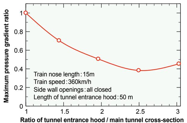
Fig. 3 Relation between tunnel entrance hood cross-section and effectiveness
