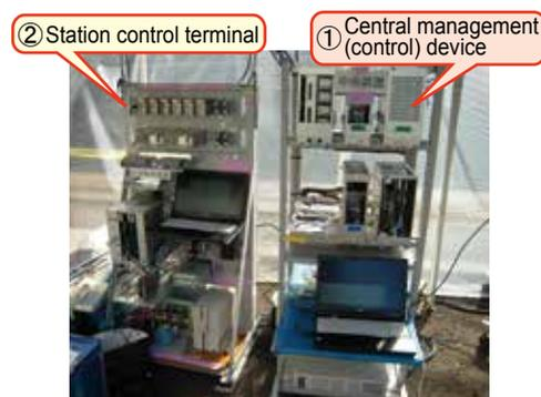
Fig. 3 Station terminal device and central management device
