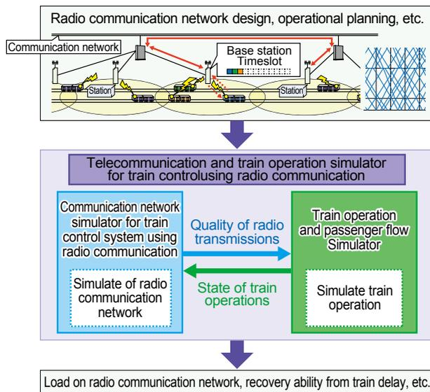
Fig. 1 Telecommunication and train operation simulator for train control using radio communication
