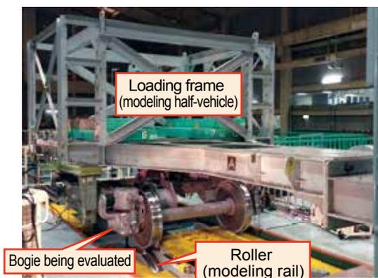
Fig. 1 Hunting tests on rolling stock test stand
