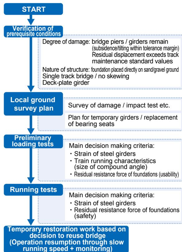
Fig. 3 Outline of flowchart supporting decision to reuse or not reuse bridge
