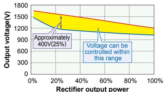
Fig. 2 Voltage control characteristics of new control method
