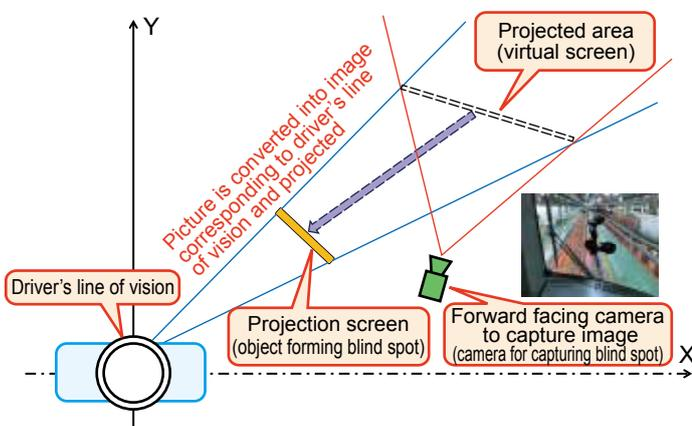
Fig. 2 Method for converting view point, by projection conversion
