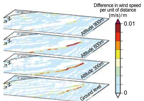
Fig. 2 Example of wind speed difference between two points about 1 km apart at each altitude whilst gusts are blowing
