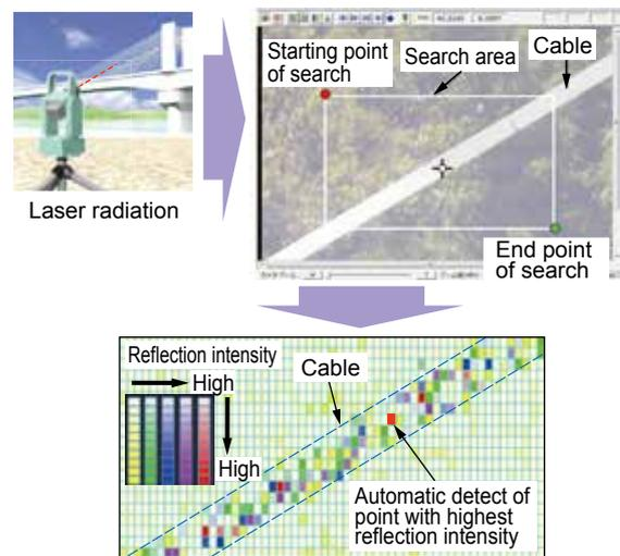
Fig. 2 Measurement cable and automatic collimation
