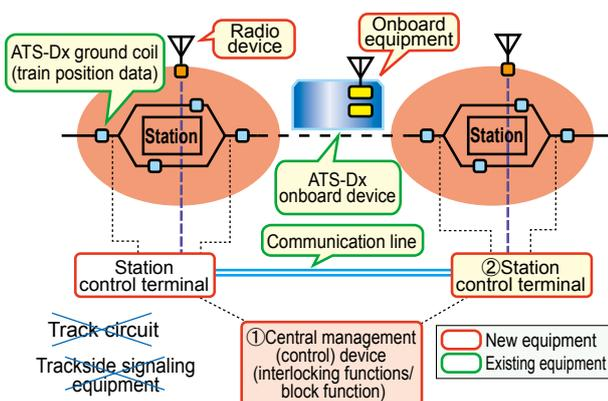
Fig. 2 Schematic of proposed new wireless train control system for regional railways
