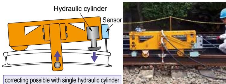
Fig. 3 Outline of automatically controlled hot rail correcting machine
