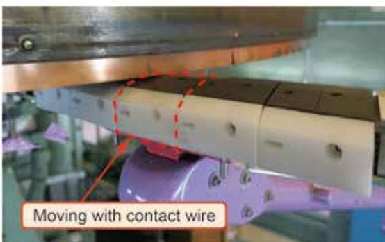
Fig. 2 Current collection performance verification tests using pantograph testing equipment
