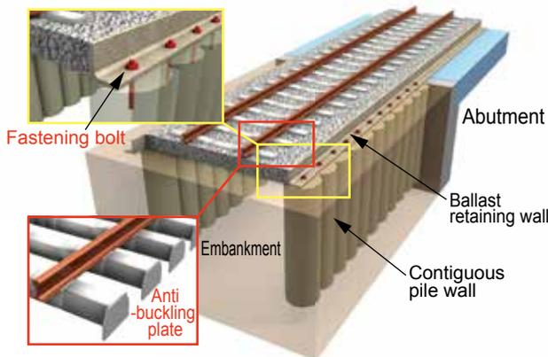
Fig. 1 Integrated ballast retaining wall and contiguous pile wall
