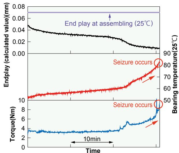
Fig. 3 Variation in bearing temperature, torque and endplay until burn-off seizure occurs
