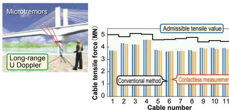
Fig. 3 Example of measurement of tensile force of cables on cable stayed bridge
