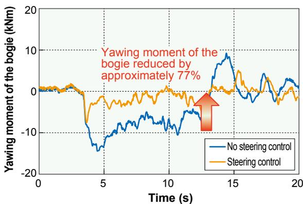
Fig. 2 Effective reduction in the yawing moment of the bogie demonstrated in bogie rotational resistance tests simulating on a curve section.
