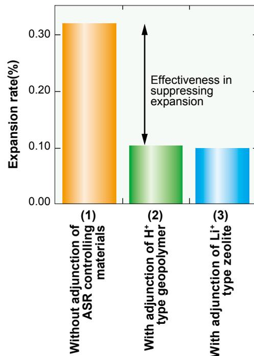
Fig. 2 Effectiveness in suppressing expansion due to ASR
