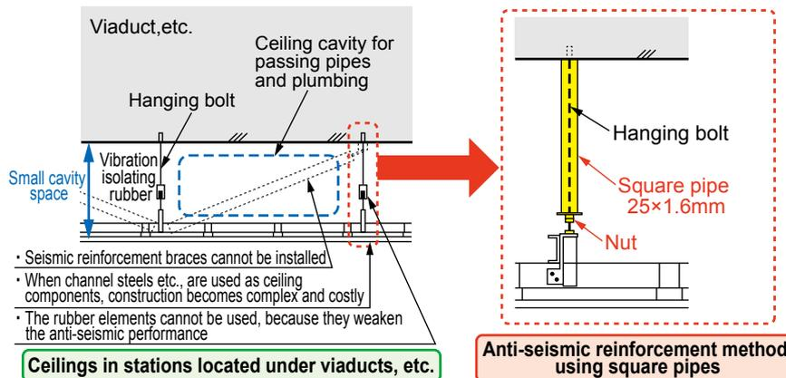
Fig. 1 Seismic reinforcement problems in station ceilings, and anti-seismic reinforcement solution using square pipe
