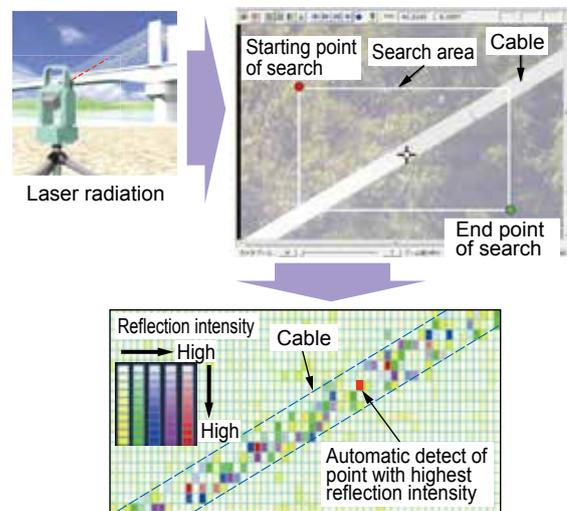
Fig. 2 Measurement cable and automatic collimation
