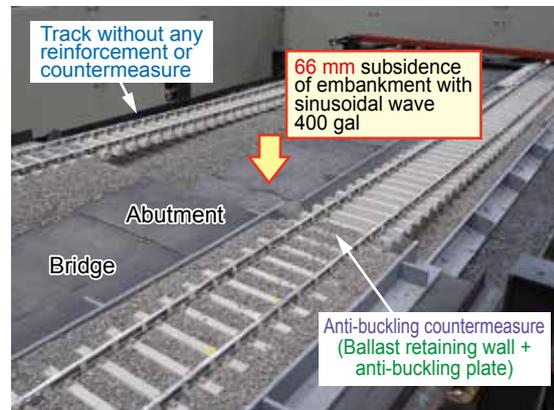
Fig. 2 Subsidence of abutment backfill without countermeasure
