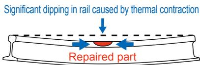
Fig. 1 Thermal contraction of repaired part
