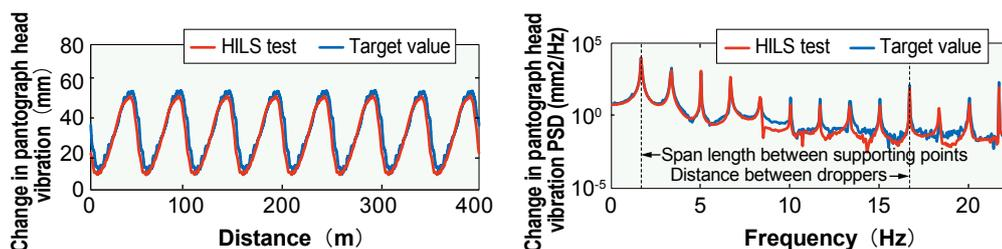
Fig. 2 Results of mock running test using HILS system (change in pantograph head vibration)
