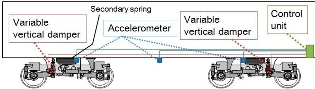
Fig.1 Structure of Vertical Vibration Reduction Control System
