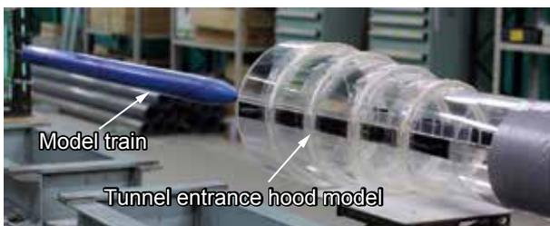
Fig. 2 Image of experiment set up for model test of tunnel hood with graduated increase in cross-section ratio
