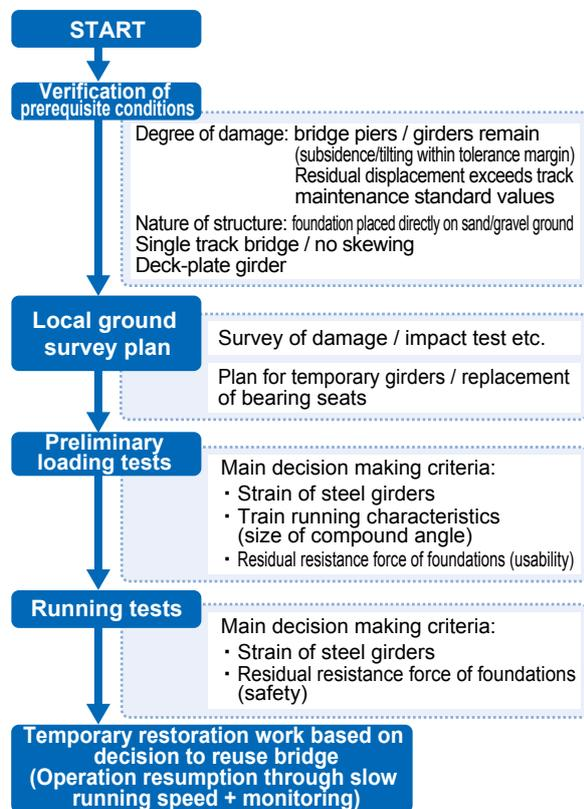
Fig. 3 Outline of flowchart supporting decision to reuse or not reuse bridge
