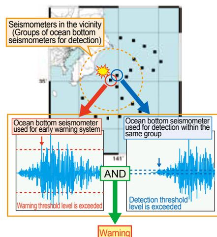
Fig. 2 Warning processing method using multiple sites
