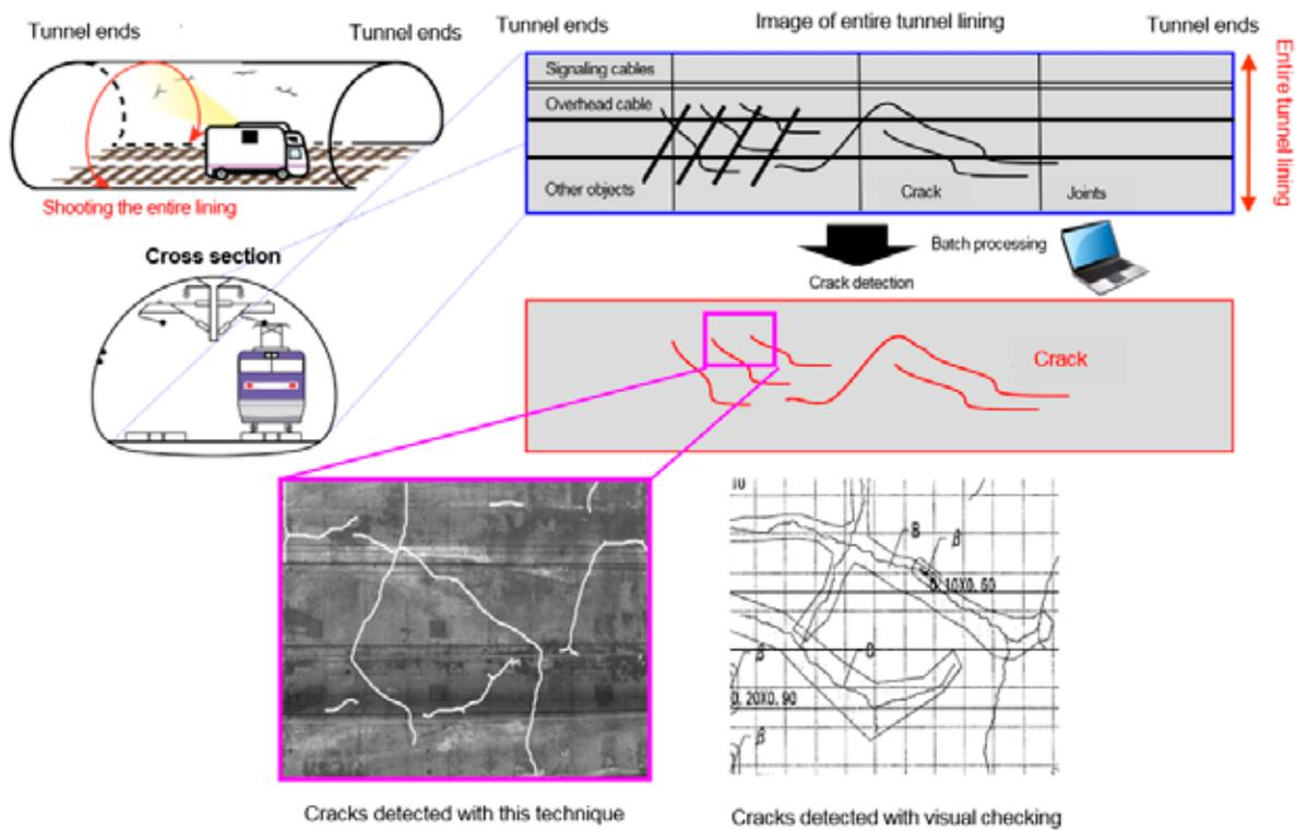
Fig.1 Cracks detected this technique
