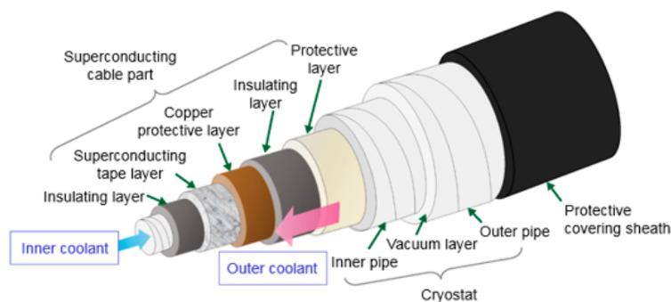
Fig. 1 Inside of Superconducting Feeder Cable
