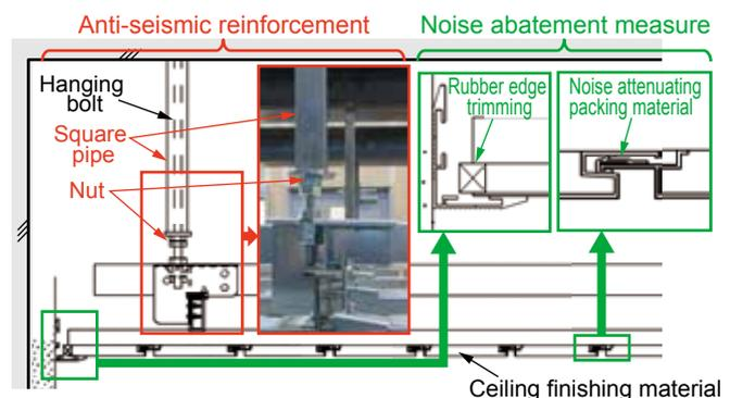
Fig. 3 Anti-seismic reinforcement method considering noise abatement
