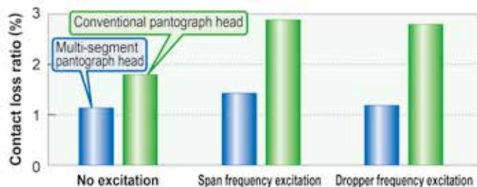
Fig. 4 Comparison of contact loss ratio between multi-segment pantograph head and conventional pantograph head
