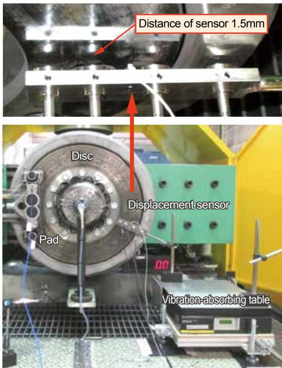
Fig. 1 External view of measuring device
