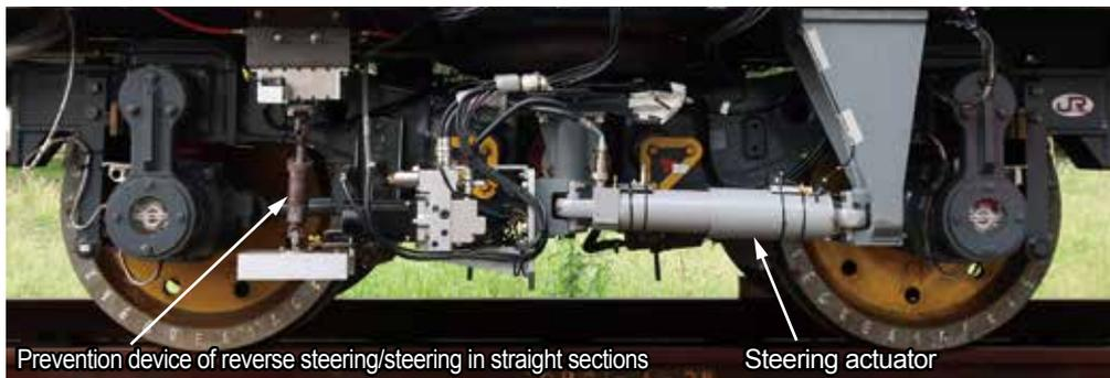
Fig. 1 Active bogie angle steering system
