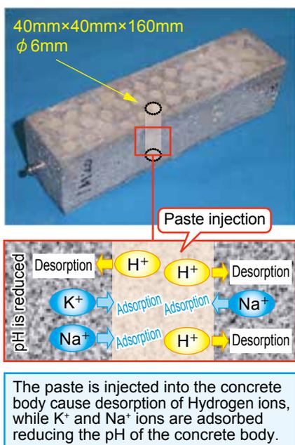
Fig. 1 Specimen reproducing grout injection into cracks and schematic showing how ASR process is suppressed
