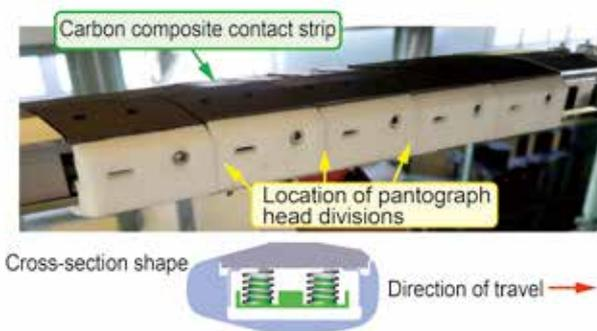
Fig. 1 Prototype of multi-segment pantograph head and cross-section shape
