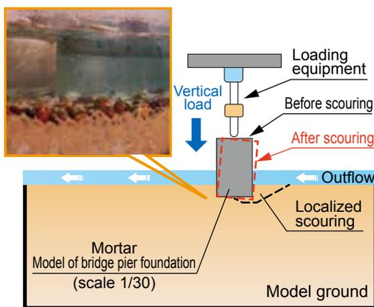
Fig. 2 Scouring test on foundations of model bridge pier
