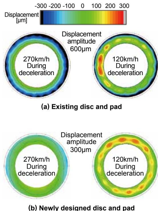
Fig. 2 Example of visualization of dynamic deformation
