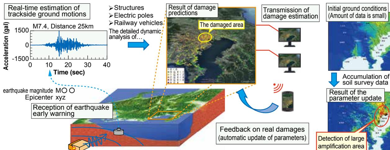
Fig. 1 Outline of earthquake damage simulator for railways
