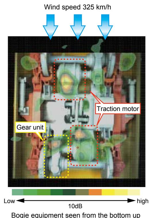
Fig. 2 Sources of aerodynamic bogie noise
