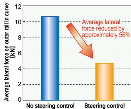
Fig. 3 Effective reduction in the average lateral force in the running tests at RTRI.
