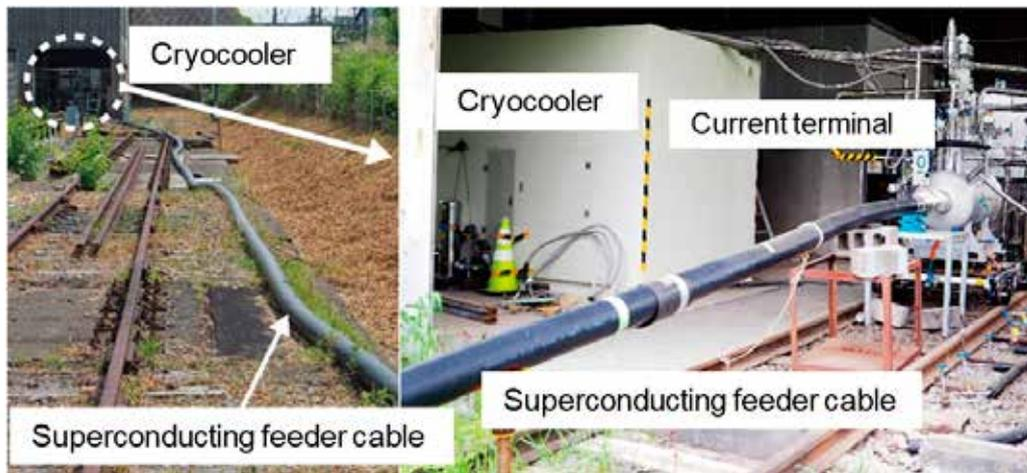
New superconducting feeder cable system at RTRI's Hino Civil Engineering Testing Station
