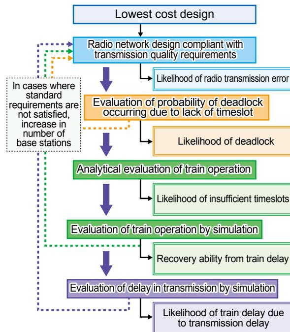
Fig. 2 Flow chart for system design
