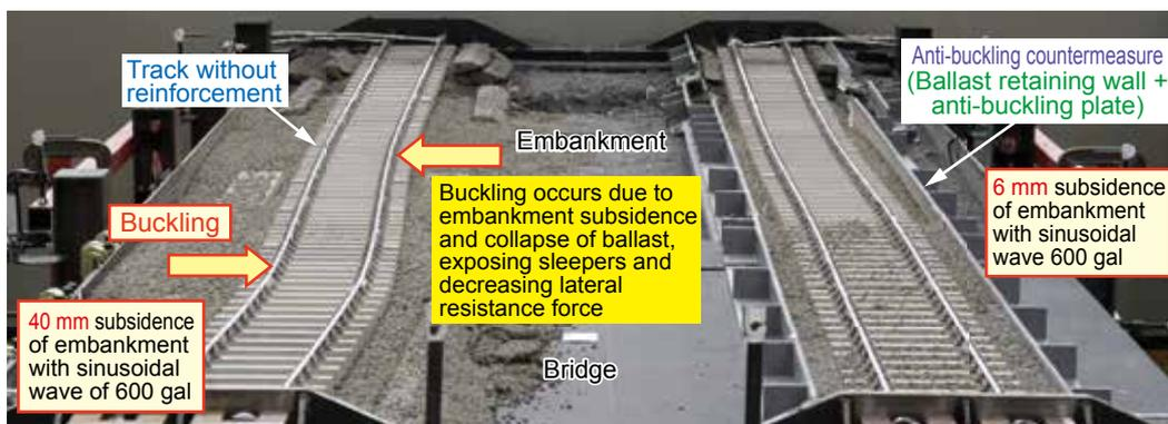
Fig. 3 Track buckling on track without reinforcement (left) and with reinforcement (right) (with reinforced embankment)
