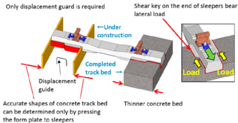
Fig.1 Newly-constructed concrete-bed track with s-shaped sleeper
