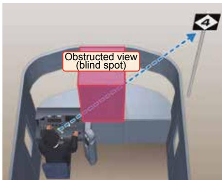
Fig. 1 Blind spot created by members in the driver's cab
