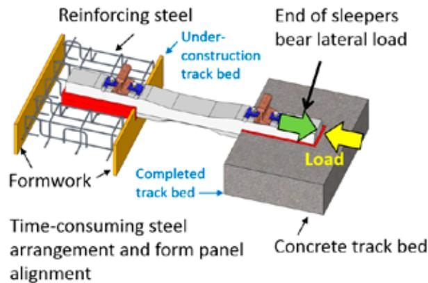
Fig.2 Existing D-shaped-sleeper concrete bed track
