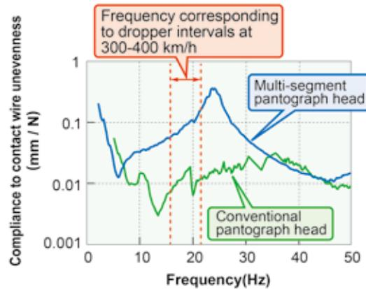
Fig. 3 Compliance characteristics of multi-segment pantograph head and conventional pantograph head
