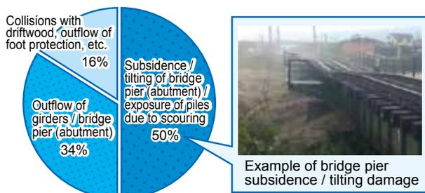
Fig. 1 Results of analysis of damage to bridge from flooding
