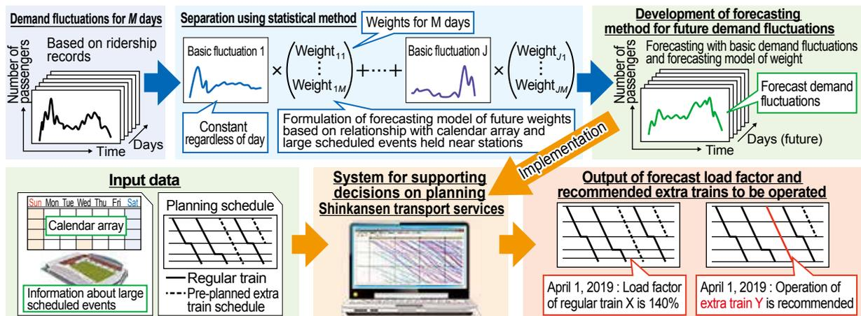
Fig. 1 Outline of the developed method for forecasting demand fluctuations and system for supporting decisions on planning transport services
