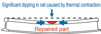
Fig. 1 Thermal contraction of repaired part
