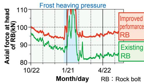
Fig. 3 Change in axial force after test work
