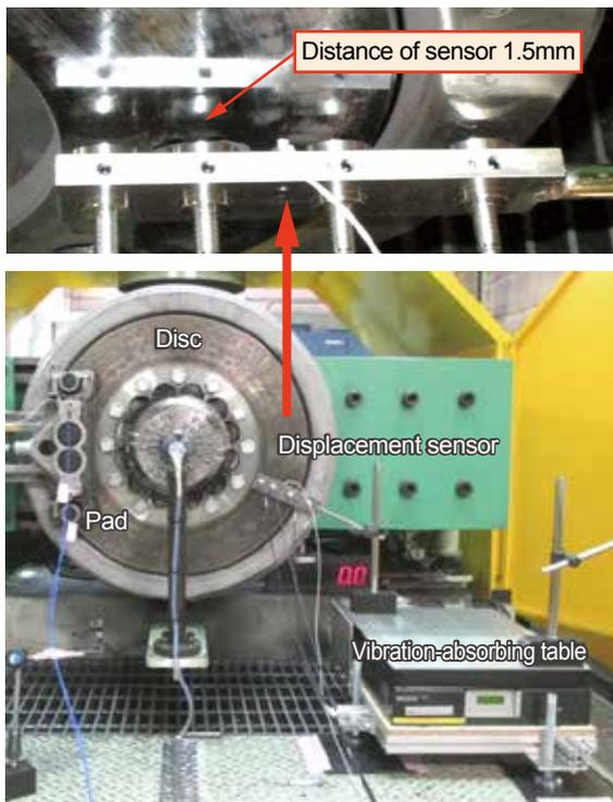
Fig. 1 External view of measuring device
