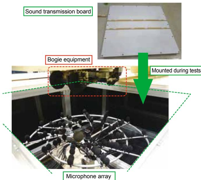
Fig. 1 Acoustic source investigation using sound
