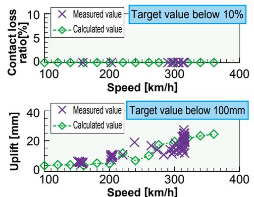
Fig. 2 In-line tests (360 km/h)
