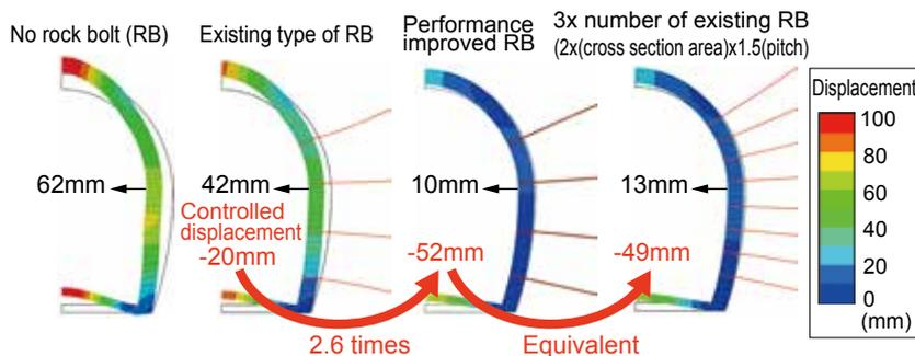
Fig. 2 Evaluation of effectiveness of displacement control through numerical analysis
