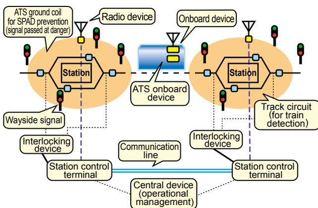
Fig. 1 Schematic of existing system (with radio communications in specific areas)
