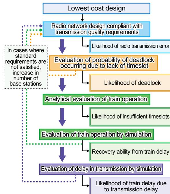
Fig. 2 Flow chart for system design
