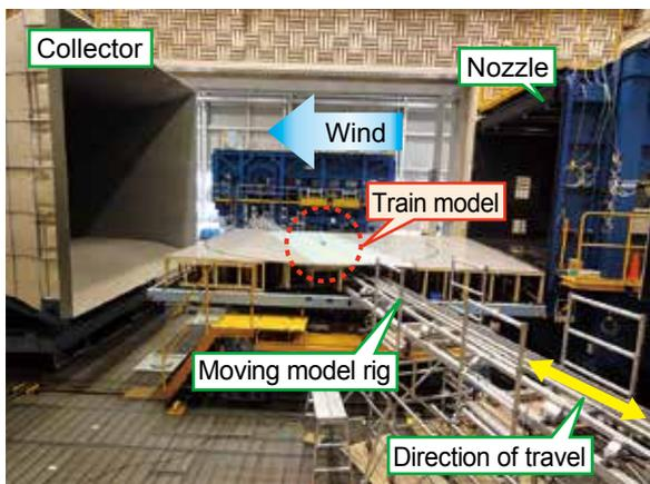
Fig. 1 View of Wind tunnel test set up (RTRI's large-scale low-noise wind tunnel)
