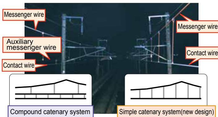
Fig. 1 Schematic and image of developed catenary system
