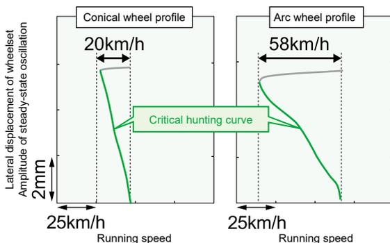
Fig. 3 Example of critical hunting curve calculation
