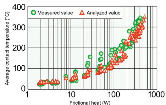
Fig. 3 Measured and analyzed values of contact temperature
