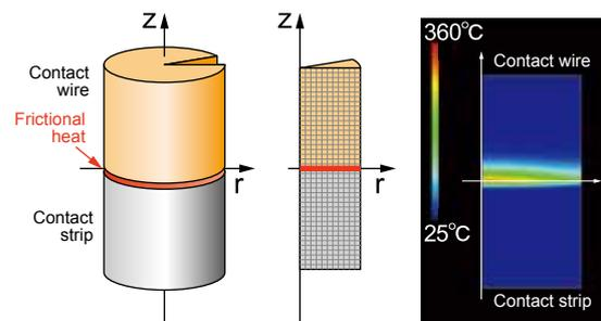
Fig. 2 Contact temperature analysis model and analysis example
