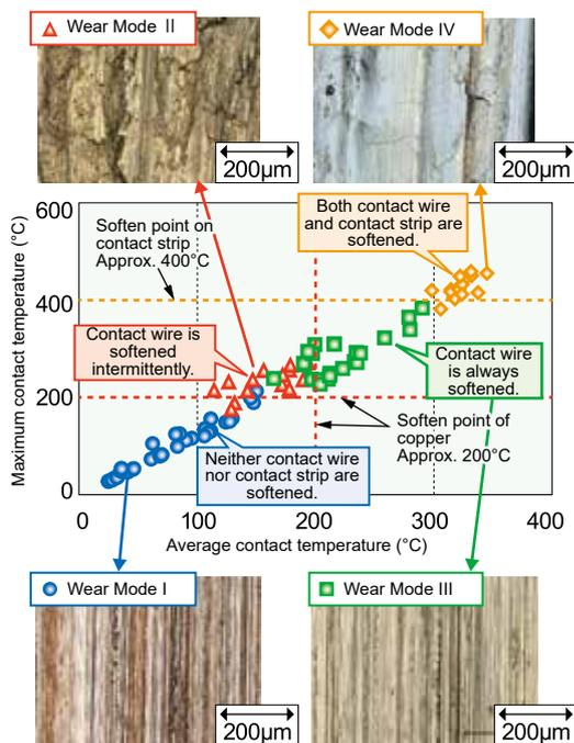
Fig. 1 Conditions for development of wear modes and wear surface on copper plate for each wear mode
