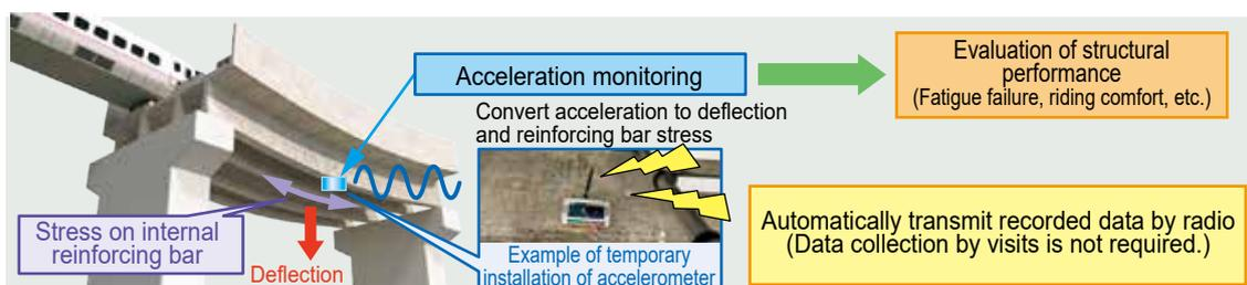
Fig. 2 Evaluation of structural performance of existing bridges by acceleration monitoring
