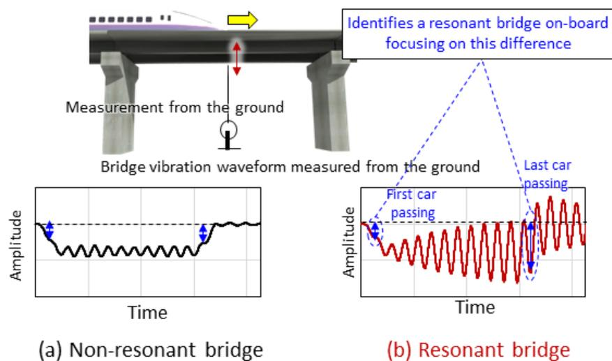
Fig.1 Vibration waveforms of ordinary (non-resonant) bridges and resonant bridges
