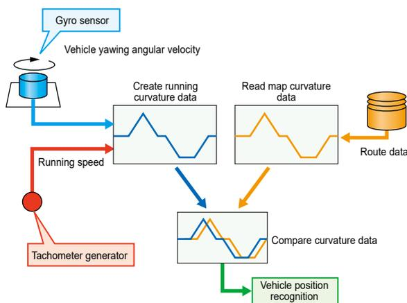
Fig. 1 Train positioning system
