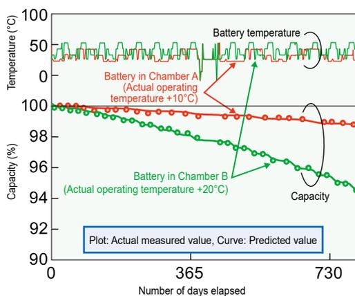
Fig. 1 Comparison of predicted values of capacity and measured values
