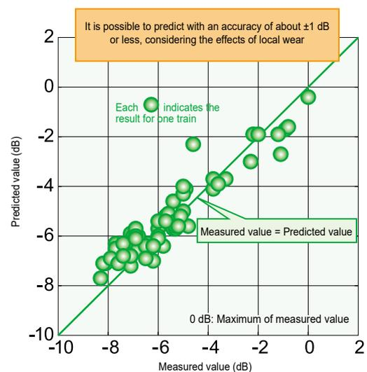
Fig. 2 Relative level comparison of measured and predicted values of wayside noises
