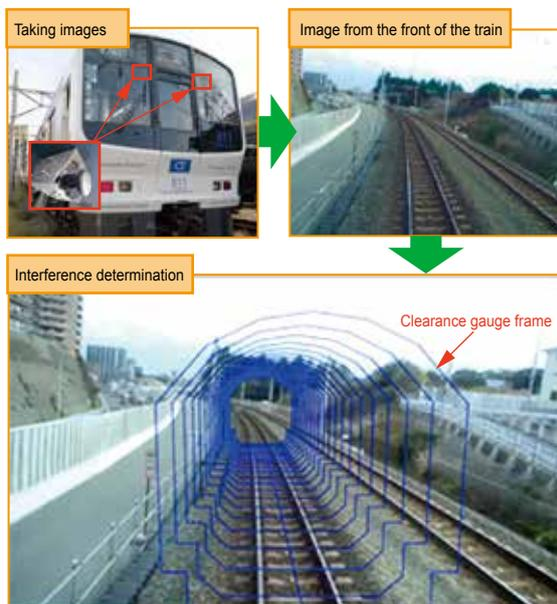
Fig. 1 Example of interference confirmation by 3D measurement
