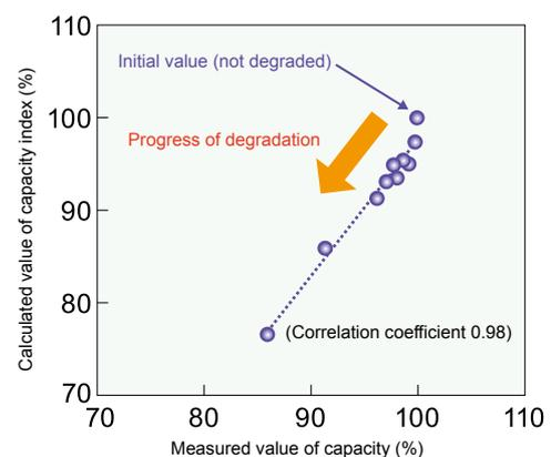
Fig. 2 Comparison of calculated values of capacity index and measured values
