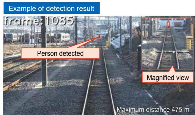
Fig. 2 Example of a person detected by the system at a distance of 475 m
