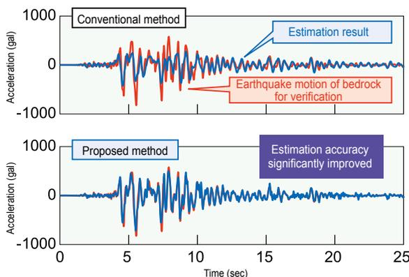
Fig. 2 Estimation results of earthquake motion of bedrock
