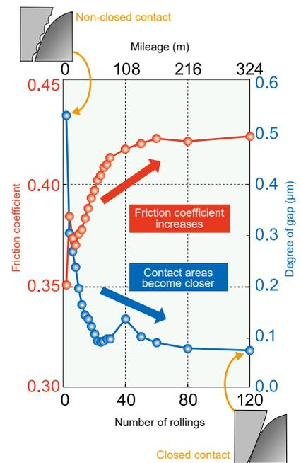
Fig. 3 Relationship between number of rollings and friction coefficient/degree of gap
