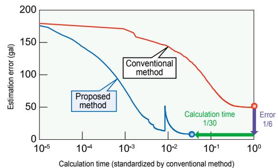
Fig. 3 Relationship between estimation error and calculation time
