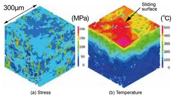
Fig. 3 Example of analysis of microscopic state distribution inside a pantograph contact strip material
