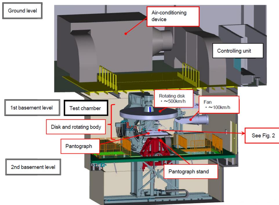
Fig. 1: High-speed pantograph testing Machine
