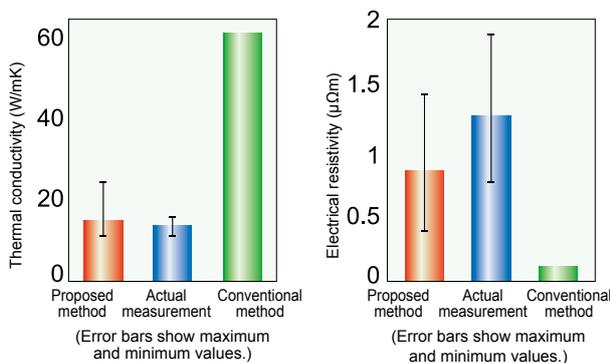
Fig. 2 Comparison of calculated and measured physical properties of pantograph contact strip materials
