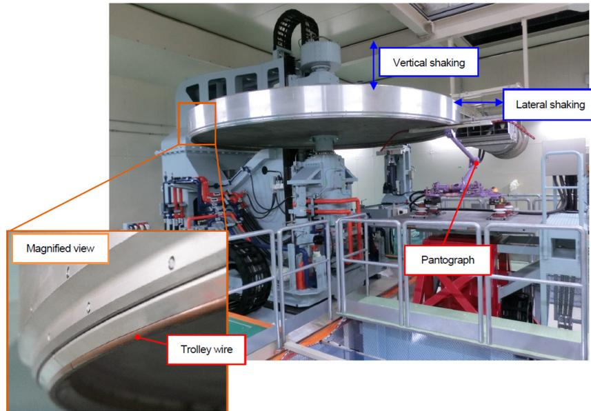
Fig.3: Rotating body and disk
