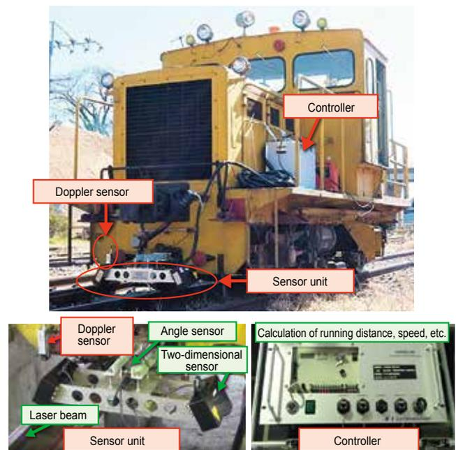
Fig. 1 Vehicle-mounted measuring device for gauge and twist under loaded condition
