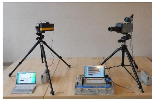
The non-contact vibration measurement system
