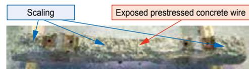
Fig. 2 PC sleeper with scaling damage
