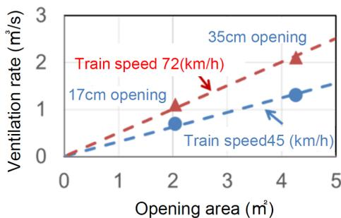
Fig. 2 Ventilation rate by opening area
