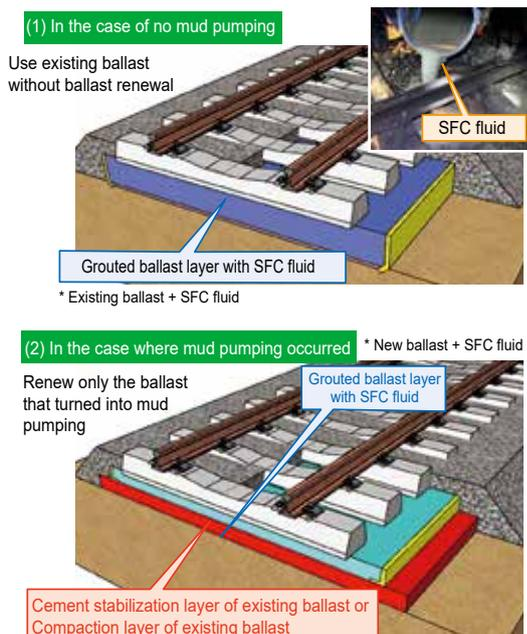
Fig. 1 Ballastless track with SFC fluid
