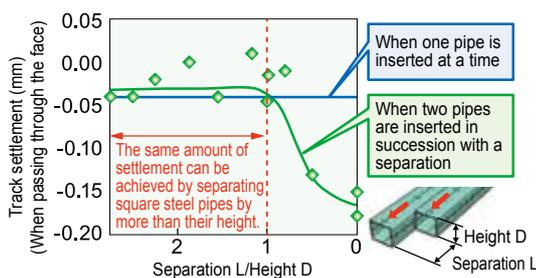
Fig. 3 Relationship between separation and track settlement
