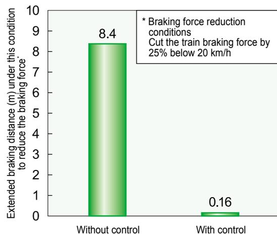
Fig. 3 Controlling braking distance extension when braking force is reduced (Running test: initial speed 30 km/h)
