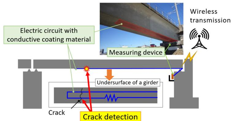
Fig.2 Crack detection system applied onto PC girders
