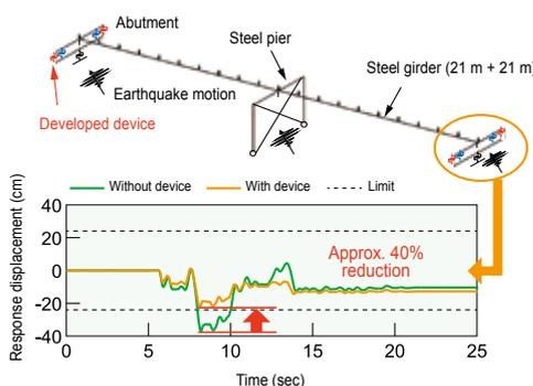
Fig. 3 Example of verification of effect by dynamic analysis
