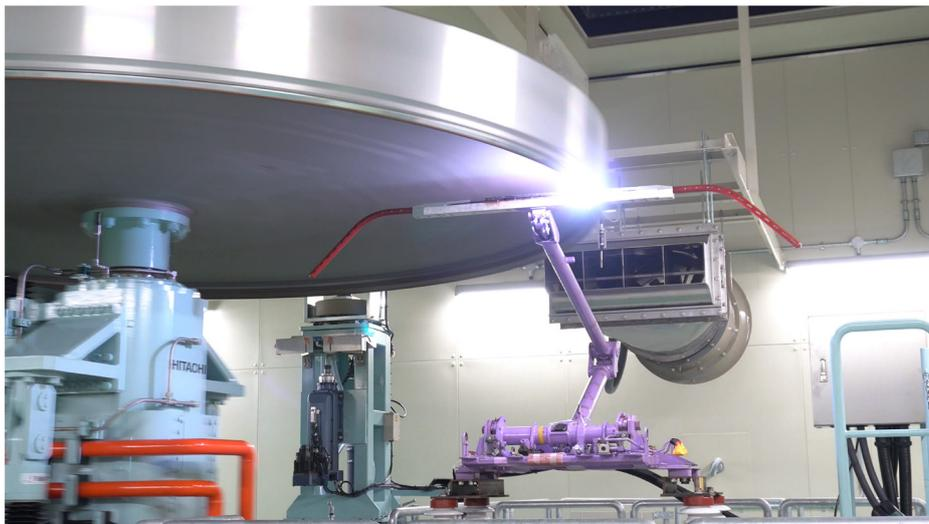
Fig.2: Testing on the high-speed pantograph testing machine
