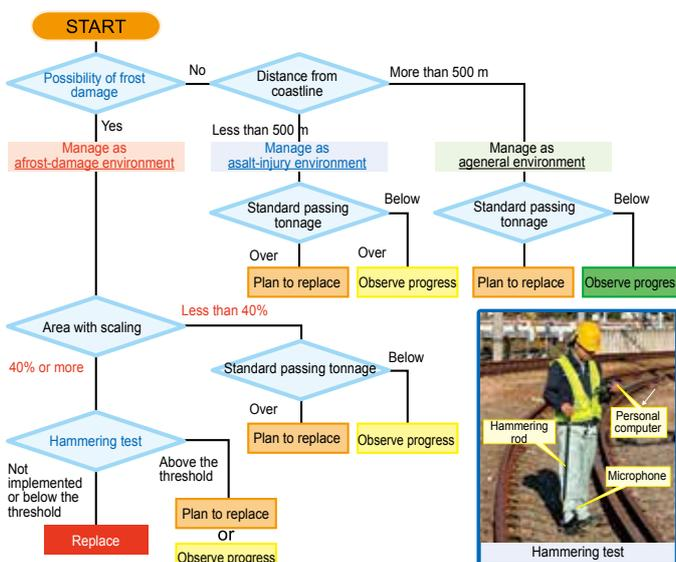
Fig. 1 PC sleeper maintenance flow
