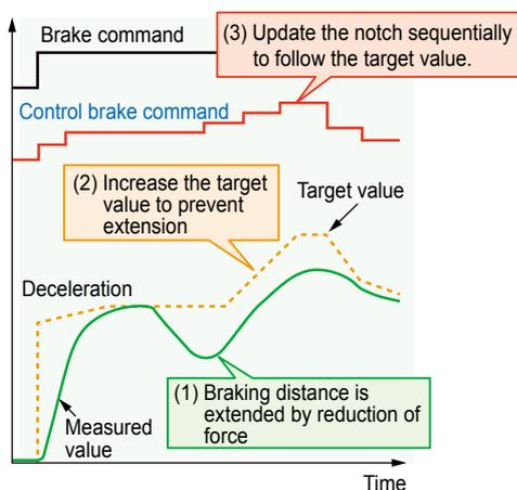
Fig. 2 Control operations of the developed method
