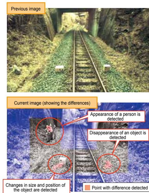
Fig. 2 Example of difference detection between images taken at two different times
