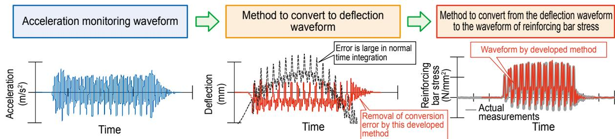
Fig. 1 Method of integrating acceleration waveform into deflection and converting deflection waveform into stress on internal reinforcing bars
