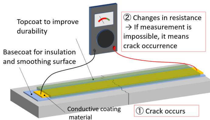
Fig.1 Crack detection with conducting coating material
