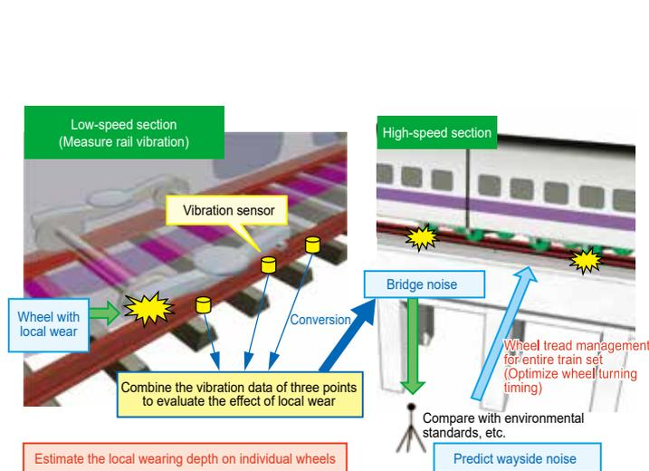
Fig. 1 Method for predicting wayside noise in a high-speed section from rail vibration in a low-speed section
