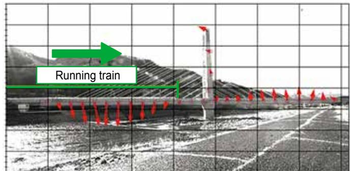
Fig. 2 Visualization of the dynamic behavior of a long span bridge when a train passes by.
