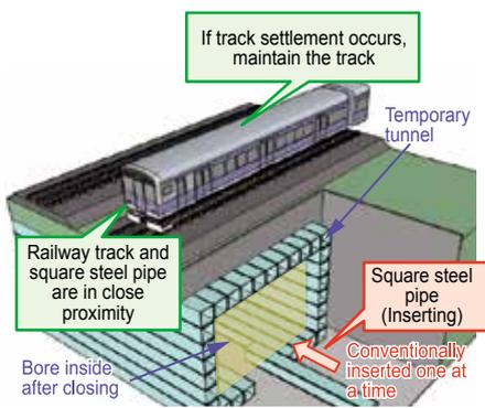
Fig. 1 Overview of constructing crossing structure under railway tracks
