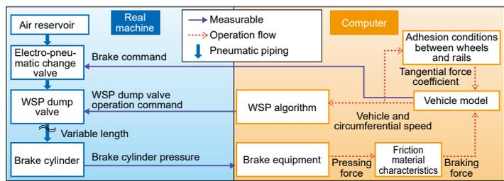
Fig. 2 Functional block diagram of WSP simulator
