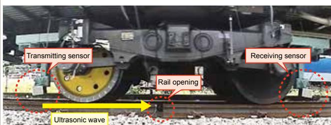
Fig. 2 Testing car equipped with sensor
