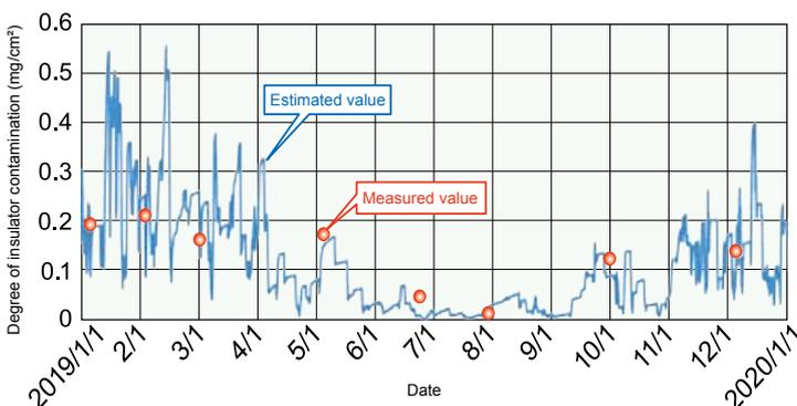
Fig. 2 Example of estimation results for the degree of contamination (on the coast of Japan Sea in Niigata)
