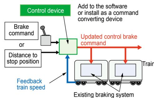
Fig. 1 System configuration of the developed method
