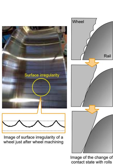
Fig. 1 Image of surface irregularity and contact state just after wheel machining
