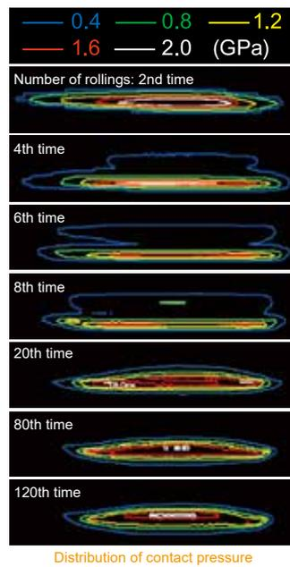
Fig. 2 Changes of contact pressure between wheel flange and rail
