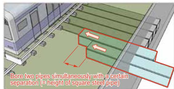
Fig. 2 Step-boring method
