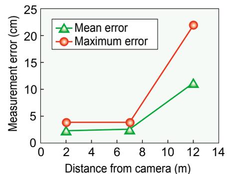
Fig. 2 Measurement errors according to distance from the camera
