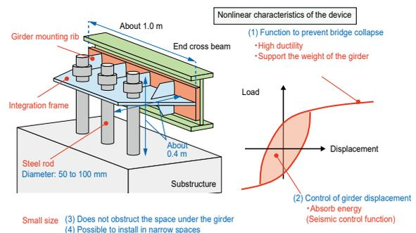
Fig. 2 Overview of the developed device
