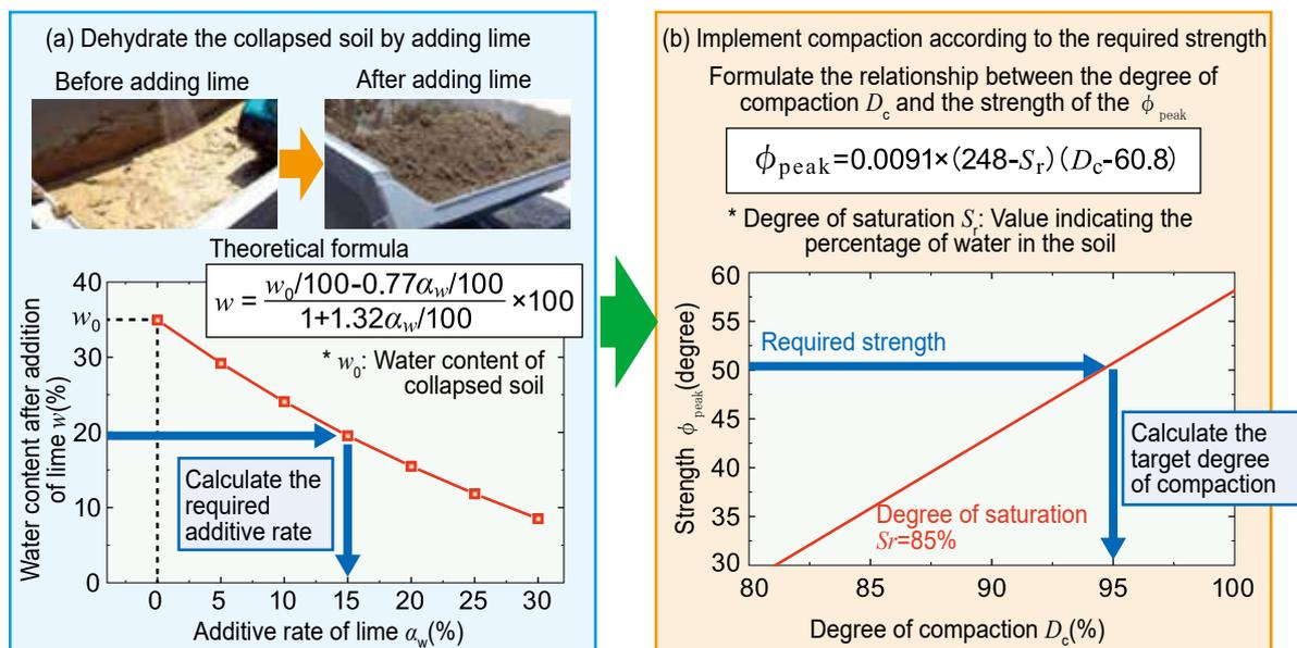
Fig. 1 Restoration method of embankments using the dehydration effect of lime and the increase in the strength of soil due to compaction
