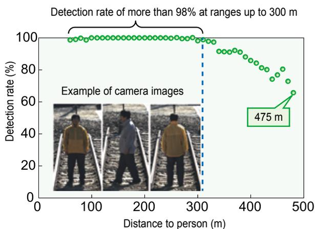
Fig. 1 Detection rate by detection distance for a person standing in daylight.
