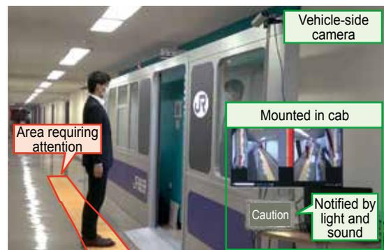
Fig. 3 Testing detection conditions using a prototype device.
