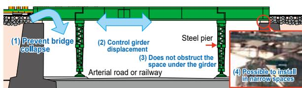
Fig. 1 Target bridge and performance requirements for the device
