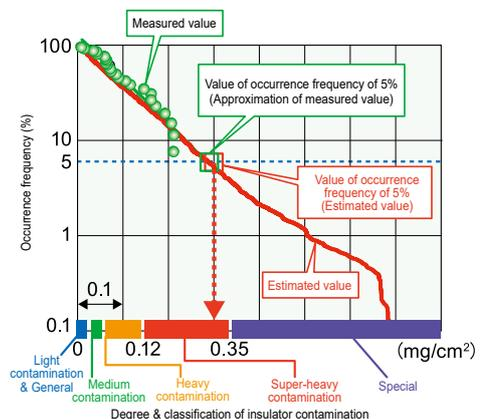
Fig. 3 Relationship between degree of insulator contamination and occurrence frequency
