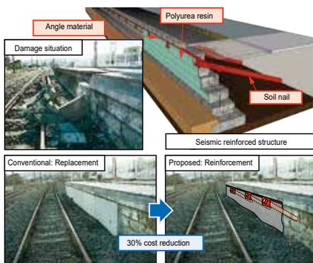
Fig. 1 Seismic reinforcement method for a masonry embankment type train platform
