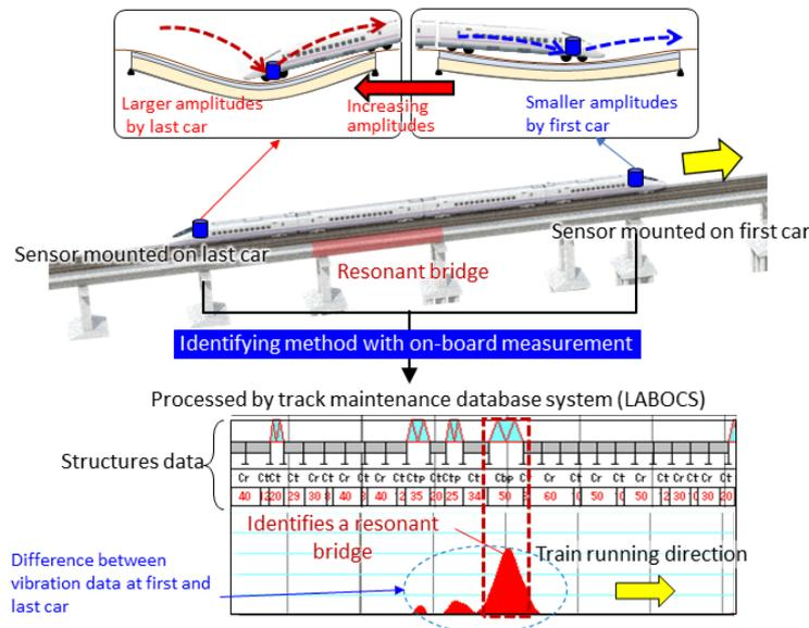
Fig. 2 The method to identify bridges that vibrates intensely using on-board measurement
