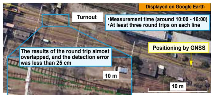
Fig. 3 High accuracy detection of measurement position by GNSS (green line)
