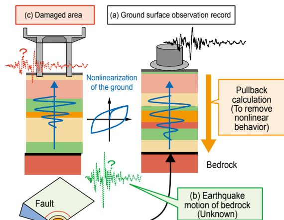
Fig. 1 Propagation of earthquake motion
