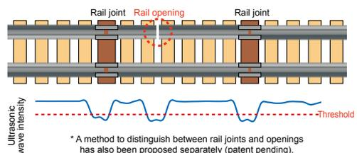
Fig. 3 Waveform when passing through a rail opening
