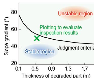
Fig. 4 Example of a nomogram for evaluating slope stability
