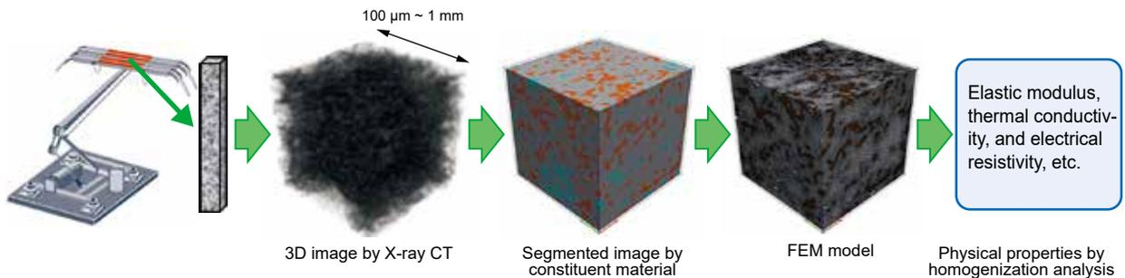
Fig. 1 Overview of the modeling of microscopic structure and physical properties evaluation method for materials
