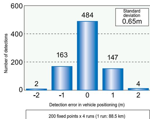
Fig. 2 Distribution of vehicle position detection errors
