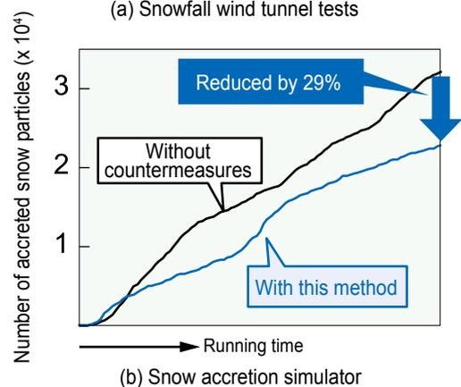
Fig. 2 Estimation of snow accretion control effect
