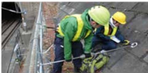
Fig. 1 Horizontal cone penetration test
