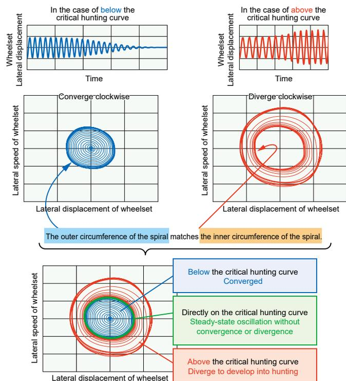
Fig. 2 Steady-state oscillation on the critical hunting curve
