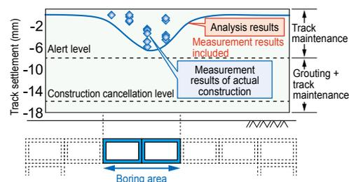
Fig. 4 Verification of the numerical analysis results of track settlement
