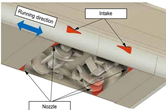
Fig. 1 Intake and nozzle layout
