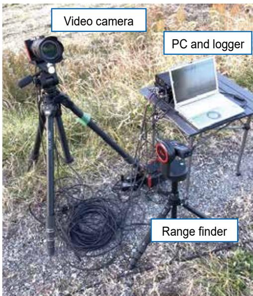
Fig. 1 Multi-point synchronous vibration measurement system using a video camera
