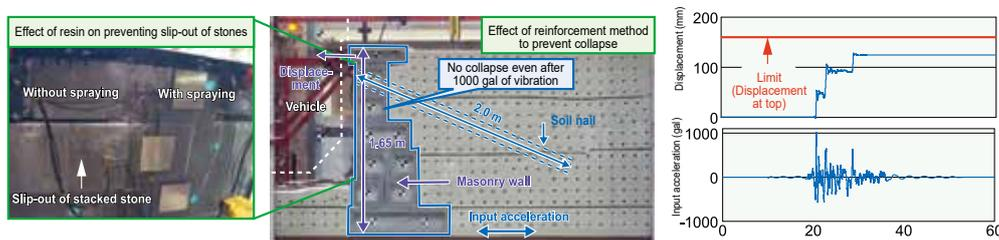
Fig. 3 Results of shaking table test using a full-scale model of a masonry embankment type train platform
