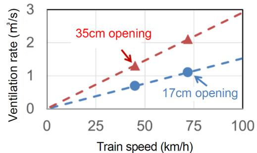
Fig. 3 Ventilation rate by train speed
