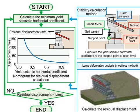
Fig. 2 Seismic reinforcement design method for a masonry embankment type train platform
