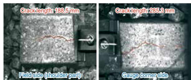
Figure 2 Example of crack extraction using the developed method
