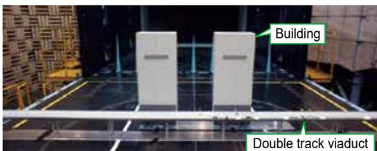
Figure 1 Wind tunnel test simulating building wind
