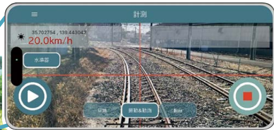
Screen shot showing the measurement screen of a train patrol support application
