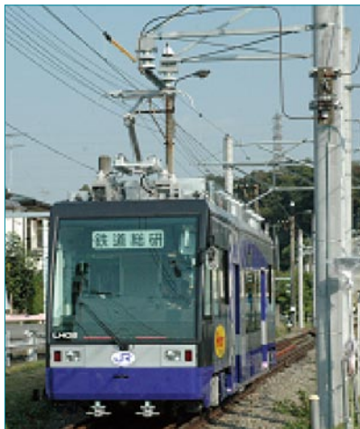
Quick charging from rigid contact wires (with a combination of sintered copper contact wires and carbon contact strips)
